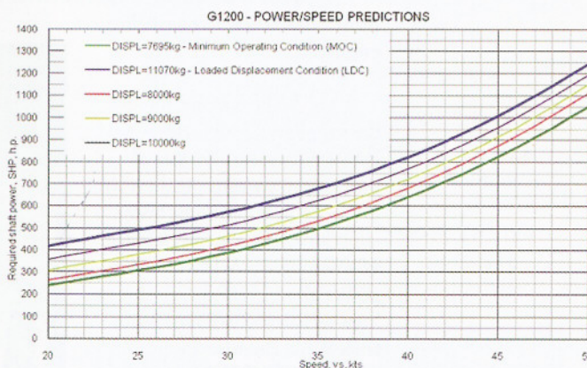
Fig.2 – Sample of speed-power predictions for 12m planning powerboat. This prediction is done by the Savitsky method, for range of displacements. Usually 2-3 different suitable methods are used for each design to get reliable predictions.
