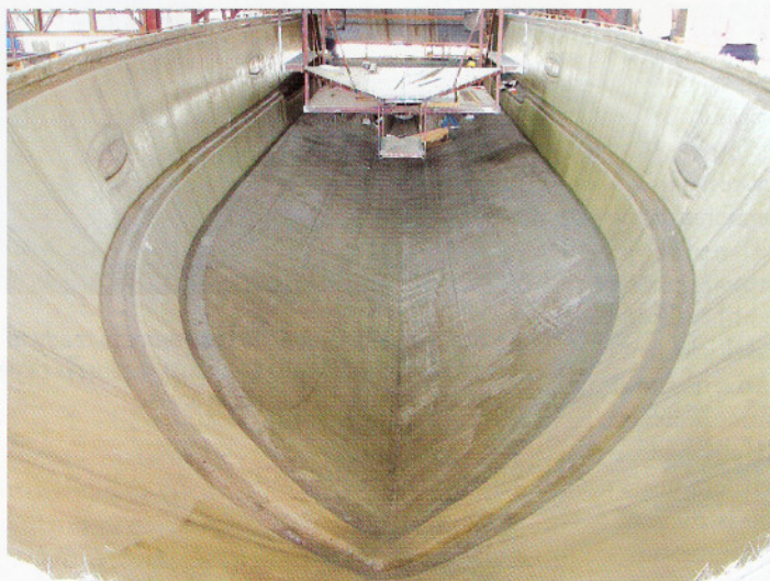
Fig.4 – Hull of 90-foot motoryacht laid in mold at SEAT Boat. This is the oldest and most established FRP boatbuilder in Thailand, delivering boats for private customers, companies and the government.
