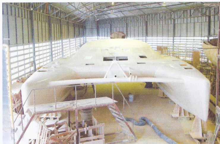
Fig.3 – Hull of Wasabi1500 catamaran in construction at RB Sailing Center. This yard is using temporary moulds built in plywood to produce such complicated shapes for custom projects.
